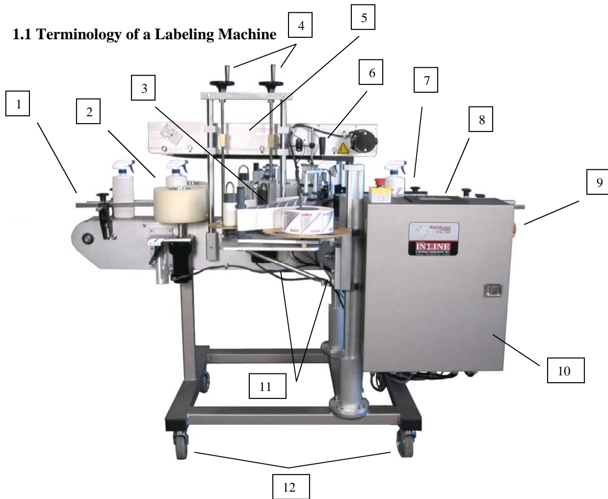
Typical Front/Back Pressure Sensitive Labeler
