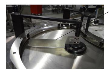
Feed Table Sweep Arm Filling Piston Nozzle Filling piston Unit.
