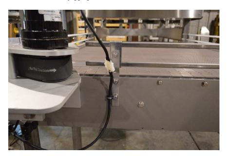
7. Connect the decline conveyor backup eye using the labeled cable.
