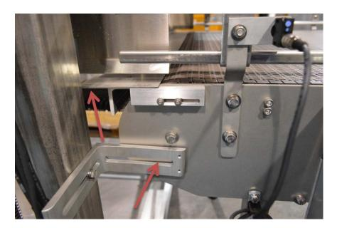
3. Attach the decline conveyor to the end of the collection table using the two supplied brackets. And level the conveyor to the discharge dead plate.
