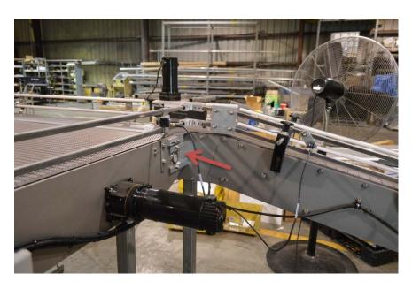
4. Using the 4 bolt bracket connect the decline conveyor rails and neck guides (if purchased).
