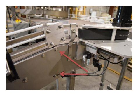
9. Connect the stack light cable, pusher and lift motor twist lock connectors.
