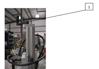
1. Cap Torqueing height Adjustment
