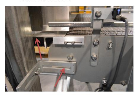
3. Attach the decline conveyor to the end of the collection table using the two supplied brackets. And level the conveyor to the discharge deadplate.
