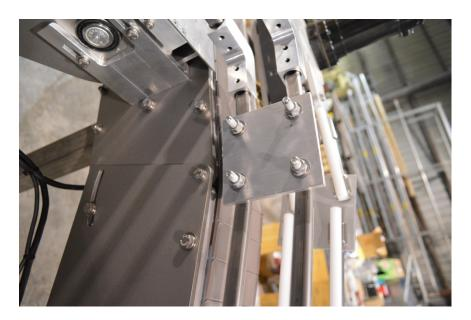
5. Connect the air supply at the quick disconnect as shown.
