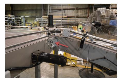
4. Using the 4 bolt bracket connect the decline conveyor rails and neck guides ( if purchased ).
